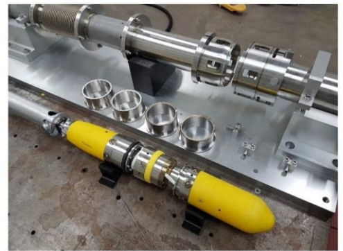
Pipe cutting rig (top), cut coupons (middle) and integrated in-bore cutting tool (bottom)
