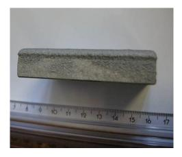
Fig. 2: Example of thick tungsten coating
