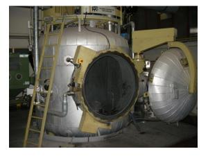
*Fig. 1: Controlled atmosphere Plasma Spray equipment*
