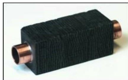
The assembled first-wall component; consisting of three graphitic heat shield blocks threaded onto the CuCrZr cooling tube, and then material-bonded via a hot isostatic pressing process
