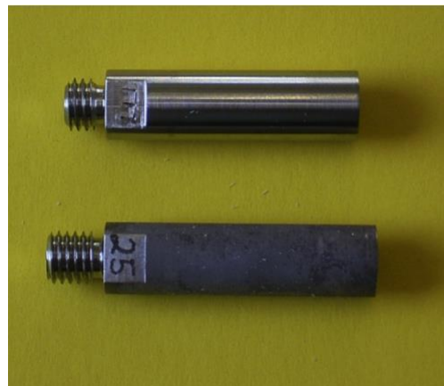
Martensitic steel component without (above) and with protective layer (below) (Source: W. Krauss, J. Konys, S--E. Wulf, O. Wedemeyer)
