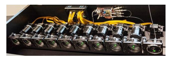
The MANTIS system collects light through a single window in the tokamak and feeds it to ten cameras that each look at a very narrow wavelength band.
