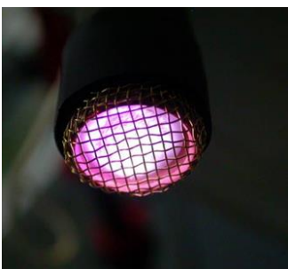
Prototypes of Radiofrequency low-temperature plasma source for biomedical and plasma medicine applications
