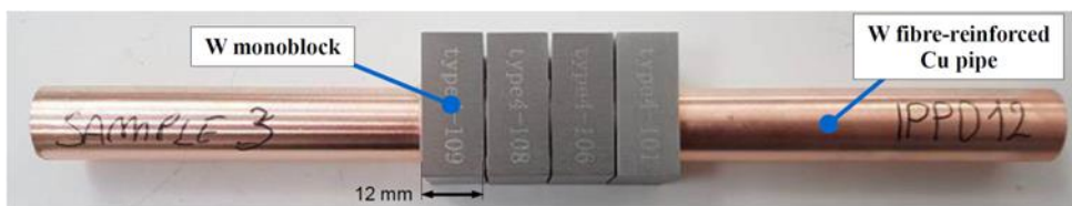
Fig.3 Plasma-facing component mock-up with Wf-Cu heat sink pipe
