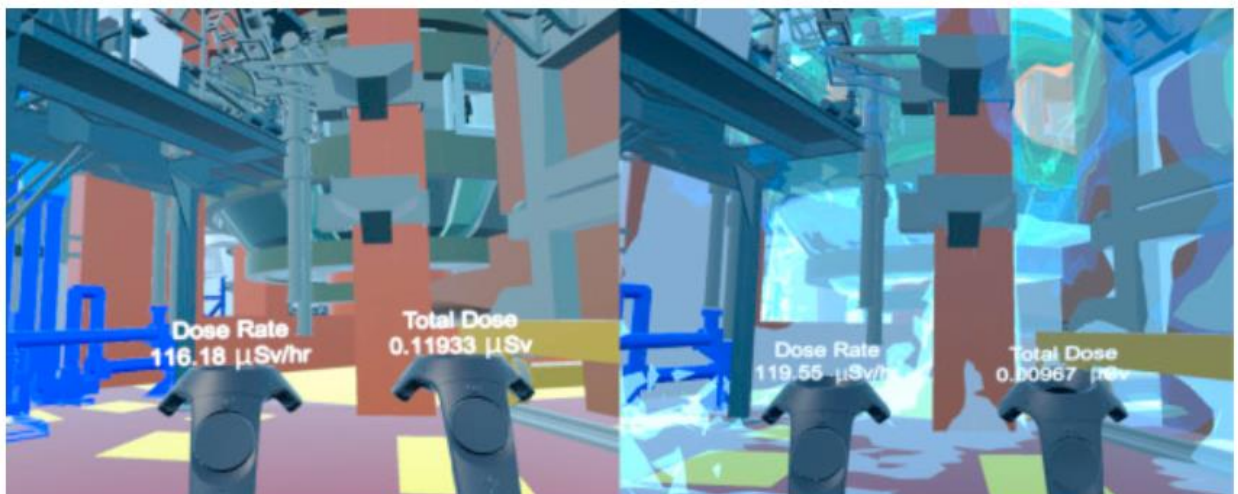
Figure 1: Screen shots taken from VORTEX inside the virtual JET model. The right image shows the radiation contours overlaid over the geometry with the colours indicating the intensity of the dose rate (UKAEA/CCFE, Culham Science Centre).
