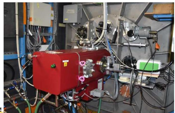
Figure 2: view of the EB gun connected to the vacuum chamber flange with all the main diagnostics dispatched around
